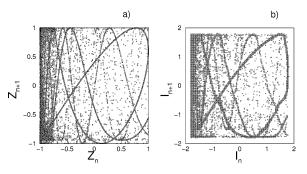
Fig. 8. Modelling versus experiment. (a) Numerical simulation of the dynamical system (23)–(25); (b) first-return map produced with the real data (current measurements) from experiments using the scheme of Fig. 6, where the circuit of the right is the one of Fig. 7(a).
