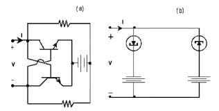
Fig. 7. Nonlinear circuits with noninvertible I-V characteristics. (a) The resistors possess  $R = 2.2 \text{ k}\Omega$ , the source voltage in the battery is 10 V and the twin transistors are 2N2222 with  $\beta = 140$ ). The I-V characteristic of this circuit is shown in Fig. 4. (b) Another circuit with a similar I-V characteristic.
