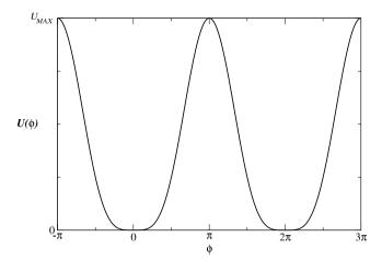
**Fig. 4.** Potential  $U(\phi) = [(1 - \cos \phi)/2]^2/2$  in Eq. (26). The kink–antikink interaction is long range for n > 1.
